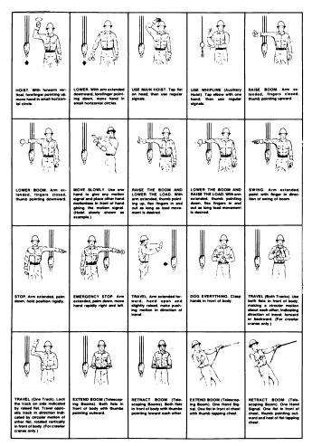
(2) The following hand signals must be used for overhead and gantry cranes and a copy must be posted in the cab at the operator's station.
